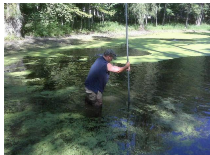
Figure 2. Taking Sediment and Water Depths
