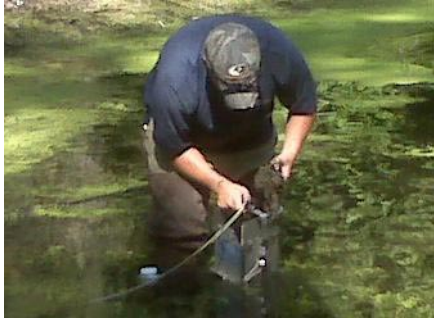
Figure 4. Putting sediment material into plastic sampling bottle
